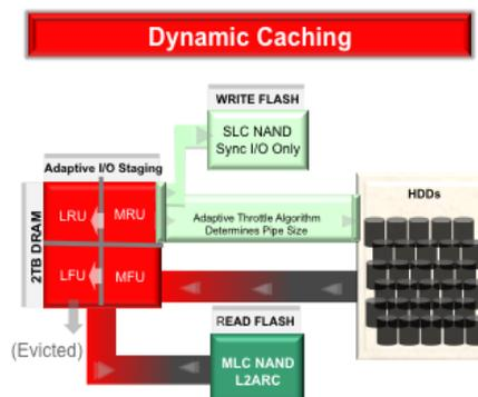
Figure 1. Hybrid Storage Pool architecture
